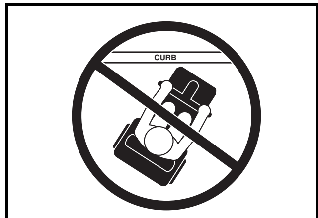
Figure 3A. Incorrect Curb Approach
