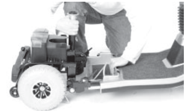
FIGURE 25. SEPARATING THE FRAME SECTIONS
