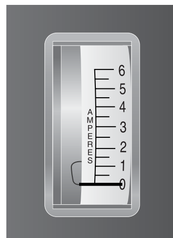
FIGURE 12. AMMETER INDICATES BATTERY IS FULLY CHARGED
