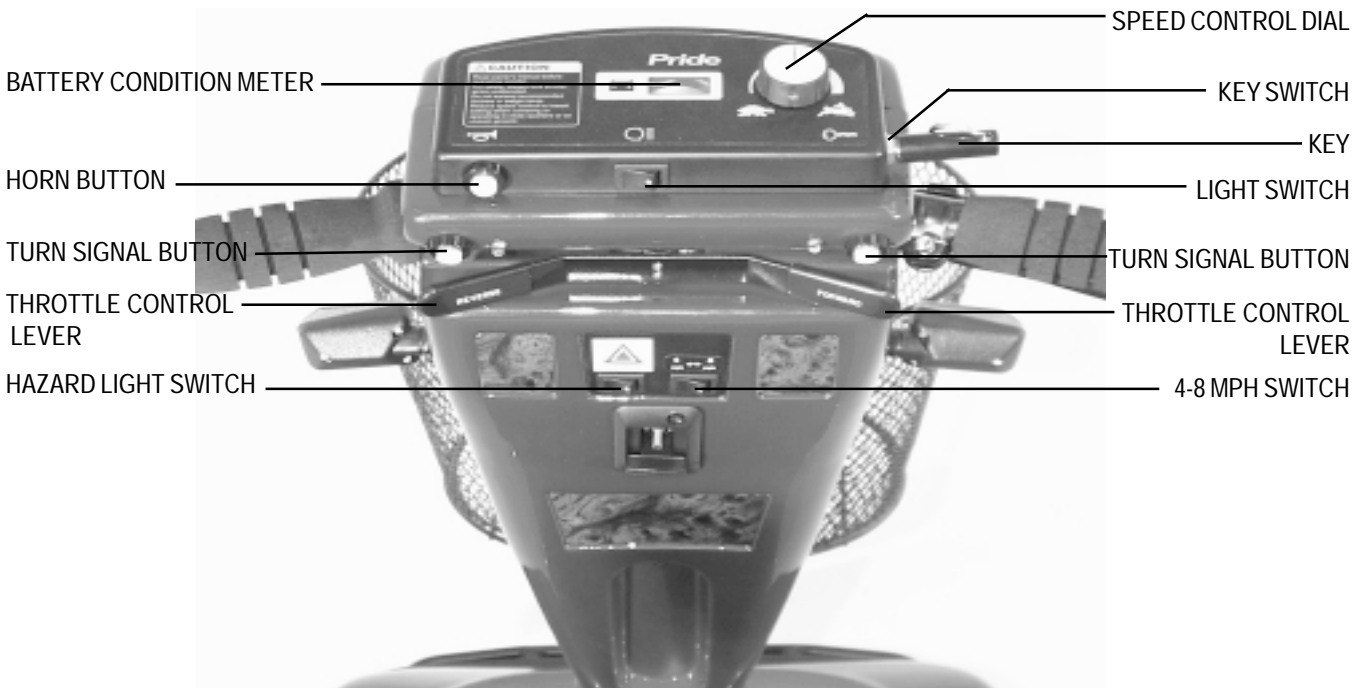
FIGURE 6. CONTROL CONSOLE ASSEMBLY
