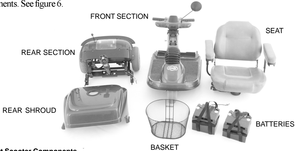
Figure 6. Sport Scooter Components
