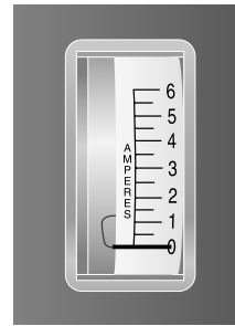
Figure 12. Ammeter Indicates Battery Is Fully Charged
