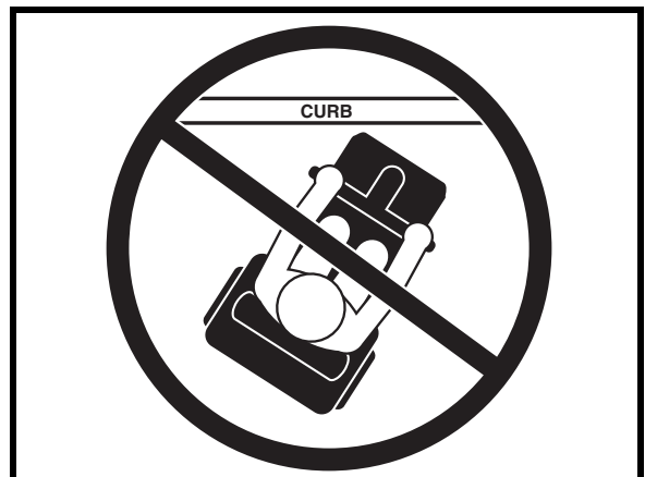
Figure 3A. Incorrect Curb Approach
