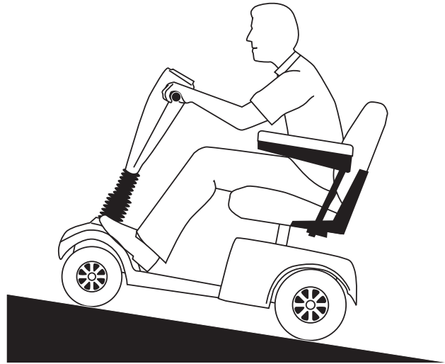
Figure 2A. Increased Stability Driving Position
