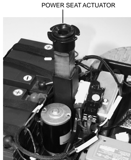
Figure 17. Power Seat Actuator (Optional)
