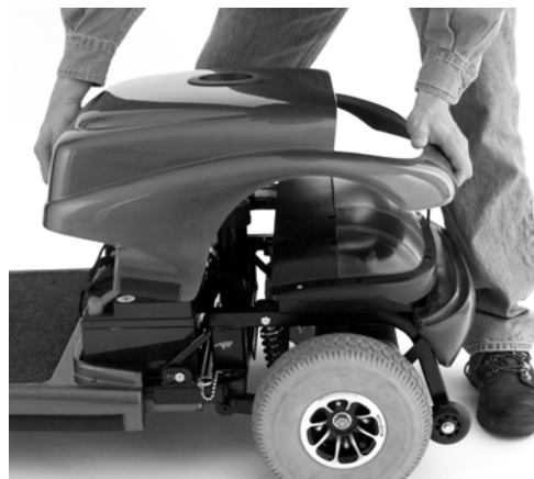
Figure 19. Rear Shroud Removal
