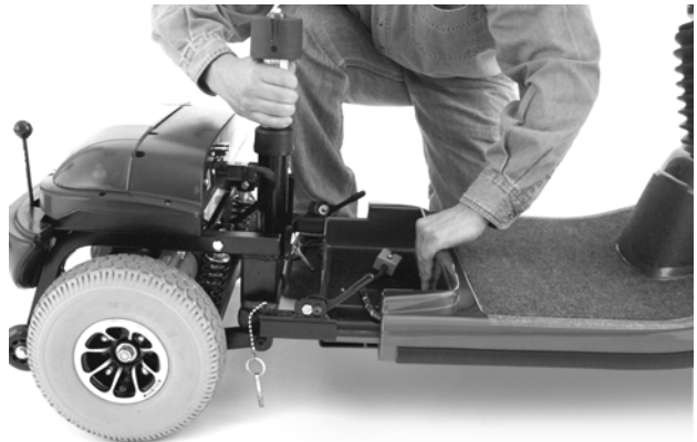
Figure 25. Separating The Frame Sections
