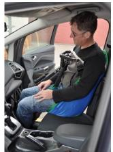
8. Lift again until the person being moved is free of the seat (Do not lift too high when inside the vehicle, as this could cause injury)
