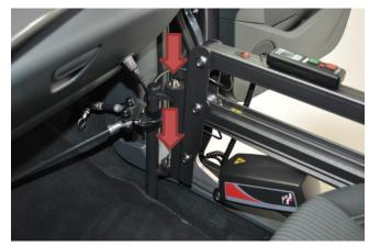
1. Mount the lift arm, extension arm and spreader bar. Rest the lower mounting lug on the longer lower pin before aligning the top pin. The arm should slide into place smoothly.
