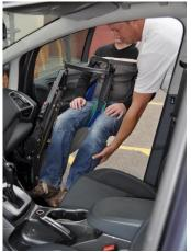
5. Using the handle on the back of the sling, maneuver the person closer to the vehicle and position their legs over the door sill, as shown above
