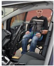
4. Raise the person off the seat (remembering to control the lateral movement manually)
