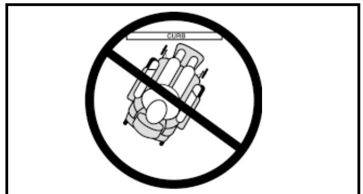
Figure 3. Incorrect Curb Approach
