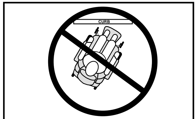
Figure 3. Incorrect Curb Approach
