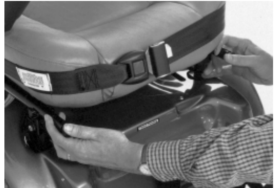
Figure 32. Removing the Seat
