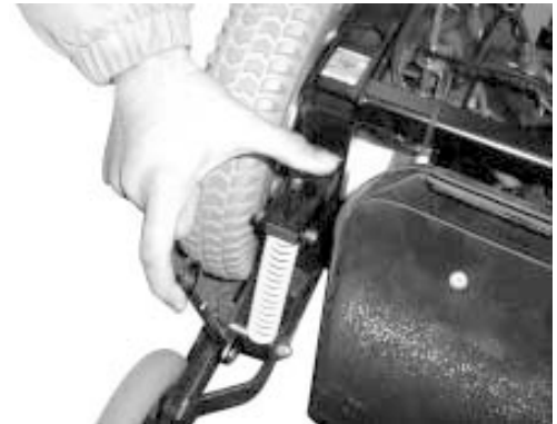
Figure 30. Anti-Tip Wheel Adjustment
