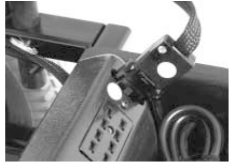
Figure 38. Charger Inhibit Plug
