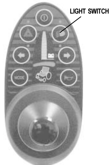
Figure 60. Full Lighting Package Light Switch
