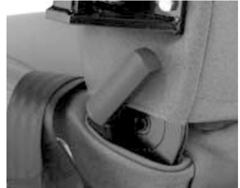
Figure 28. Seatback Release Lever
