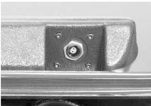
Figure 3. Remote Plus Controller Harness Connector
