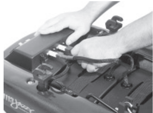
Figure 34. Disconnecting Battery Box Connections
