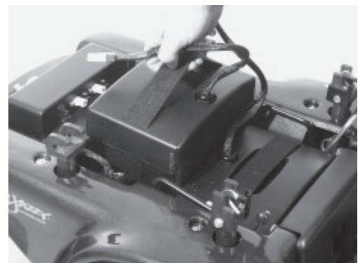
Figure 35. Battery Box Removal
