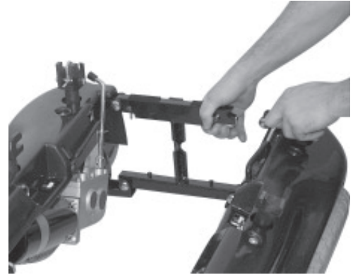
Figure 20. Fitting the Frames
