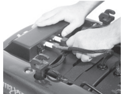
Figure 8. Disconnect Battery Cases
