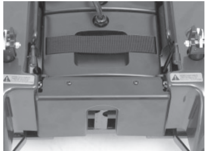
Figure 3b. Drive Motors Engaged.
