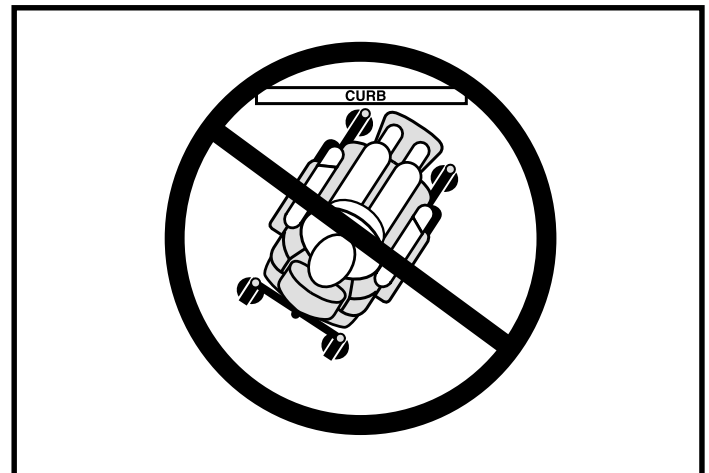
Figure 3. Incorrect Curb Approach
