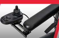
Optional swing-away joystick swings out at an angle for convenient access
